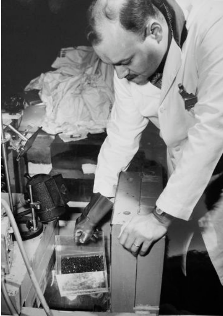
Figure 5.3. A Brookhaven biologist places a lucite box containing seeds into the thermal exposure facility at the Brookhaven nuclear reactor. This “thermal column” enabled the biologists to expose materials to thermal neutron bombardment without interrupting the operation of the reactor. Papers of W. Ralph Singleton, Albert and Shirley Small Special Collections Library, University of Virginia.
